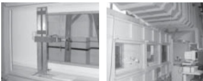
(Left): Inside the test section: A Micro-UAV Engine (Right): Inlet side of the test section and lower half of upper diffuser
