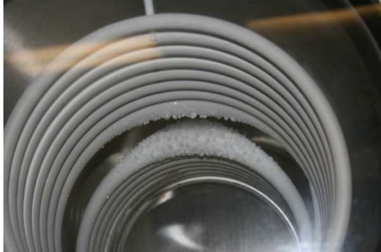
FIGURE 1. Photograph of the Coils in a Lyostar II Condenser with non-uniform ice buildup
