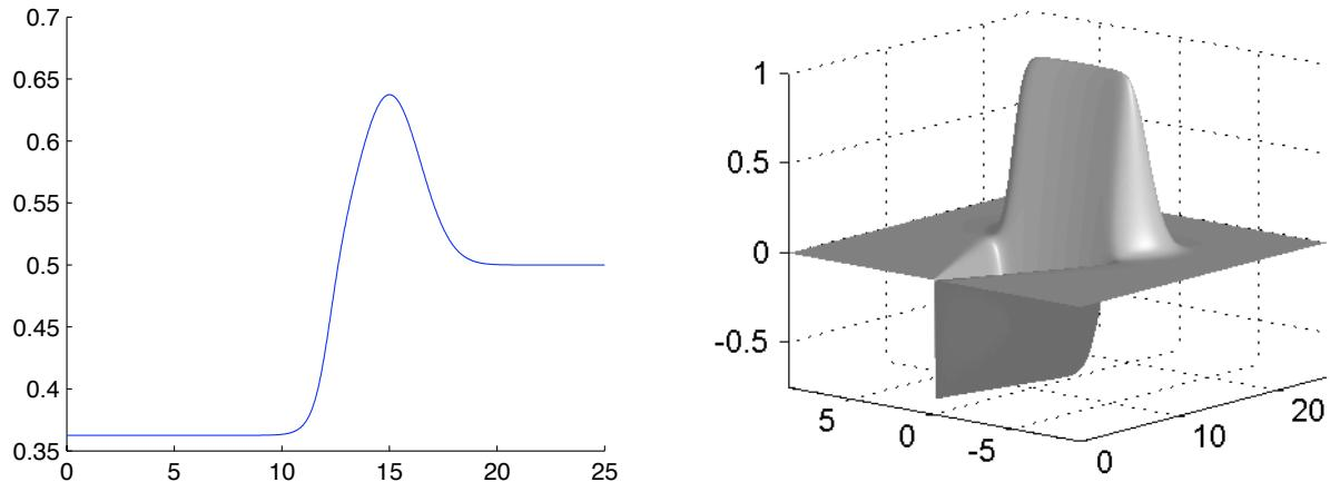
(a) Range vs. probability for  $r^* = 15$  and  $\sigma_r^2 = 2$ . Note the comparatively low probability of occupancy for  $r < r^*$ .
