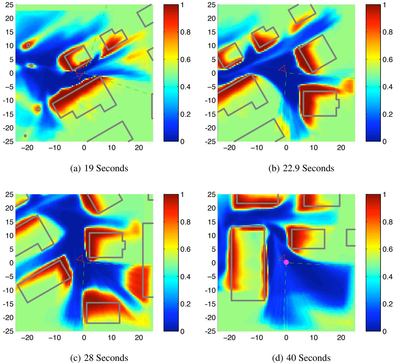
**Fig. 8** Sequence of images from representative run. The vehicle is shown as a red cranked triangle, camera field of view is shown as green dashed lines. Red represents a high probability that a cell is occupied; blue represents a low probability that a cell is occupied (i.e. high probability that the space is free). Green represents a 50% probability (uncertainty) that a cell is occupied. Obstacles are shown as gray lines, the magenta dot is the goal.
