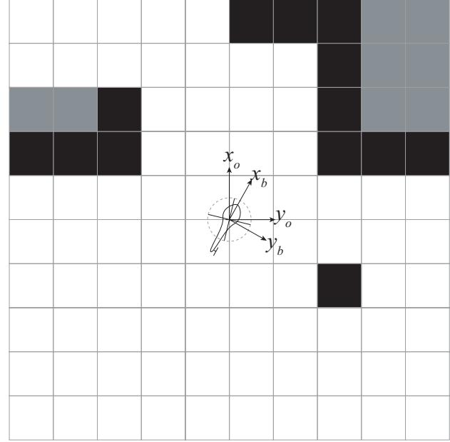
**Fig. 3** Schematic of occupancy grid. Cells which are known to be free are white, those which are known to be occupied are black, those which are unknown are grey. Coordinate frames and the vehicle are shown at the origin of the grid.
