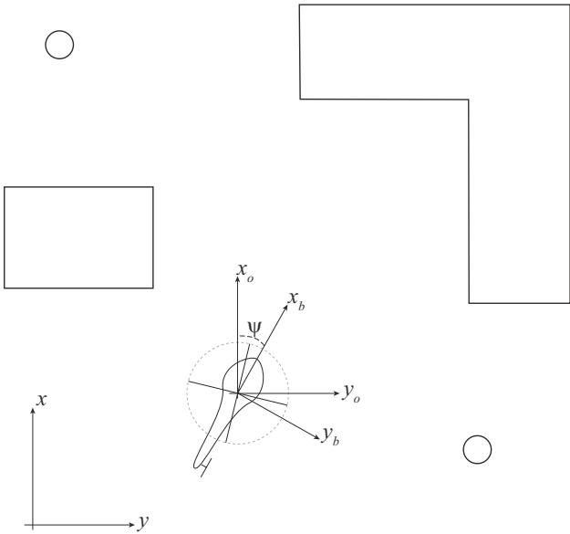
**Fig. 1** Navigation/avoidance scenario. The autonomous rotor craft must fly to a goal (not shown) while avoiding small, convex obstacles (e.g. tree trunks) as well as large, potentially non-convex obstacles such as buildings.
