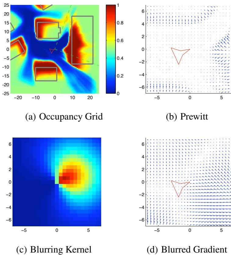
**Fig. 6** Creating the potential field due to the occupancy grid at 31.1 seconds. Subfigures (a) and (c) use the same color bar. The vehicle is shown by the cranked triangle. Motion is upwards to the right.
